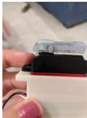
Figure 17: Servo Motor End Effector with Silicone Coating
