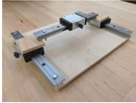
Figure 3: Base Plate with three Sliding Rails and Carriages
