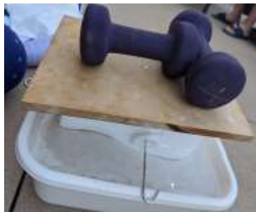
Figure 15: Styrofoam Head pushed into Mold with Liquid Silicone
