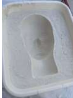
Figure 13: Completed Plaster Mold
