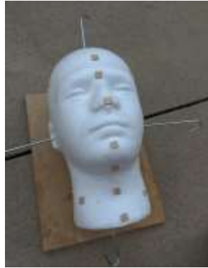
Figure 14: Styrofoam Head with Spacers
