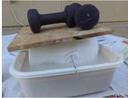
Figure 12: Styrofoam Head inserted into Wet Plaster
